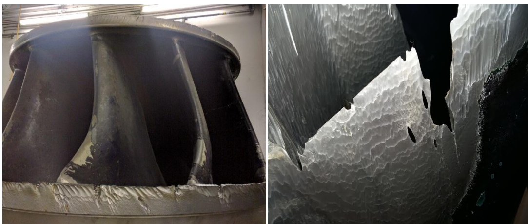
Figure 2-9: Wear and tear in turbine components (Source: NEA, 2016 b)
