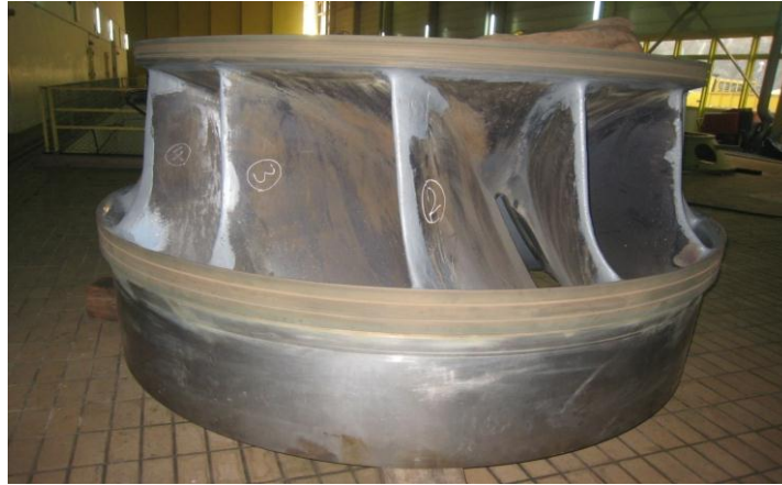
Figure 2-2: Turbine Erosion (Source: NEA, 2016 a)
